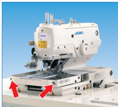
Material opening amount adjusting screw
