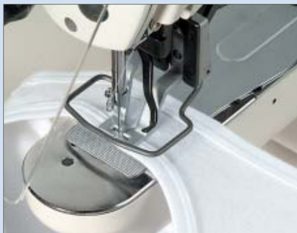
❖ M type (Bartacking shoulder of running shirt)
