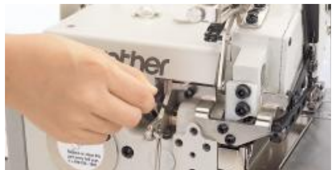
Adjusting upper feed vertical amount
